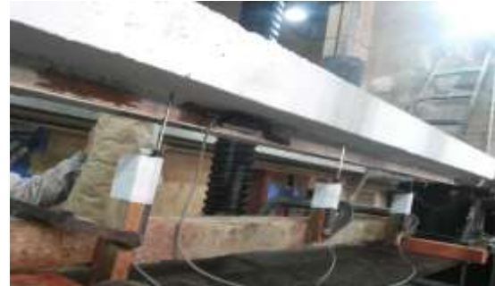
Figure (4): Vertical deflection measurement.
