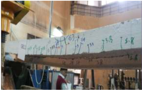
Figure (8): Crack pattern of composite beam GB1.1.
