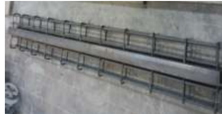
Figure (1): reinforcement of tested composite beams
