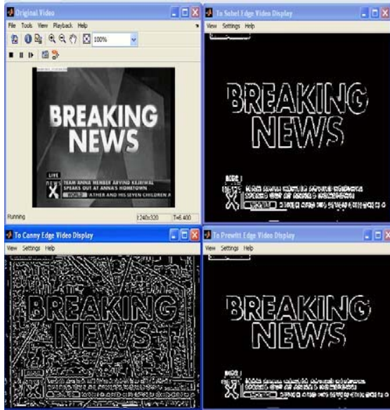
Fig.5: a) Original b) Prewitt c) Sobel d) Canny.
