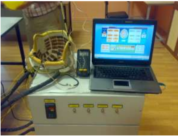
Figure 6. No load test assembly of brain cooler
