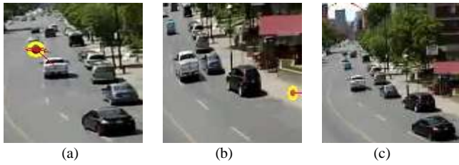
Figure 3. Tracking captures of second video: (a) Proposed tracker; (b) Condensation tracker; (c) Camshift tracker.
