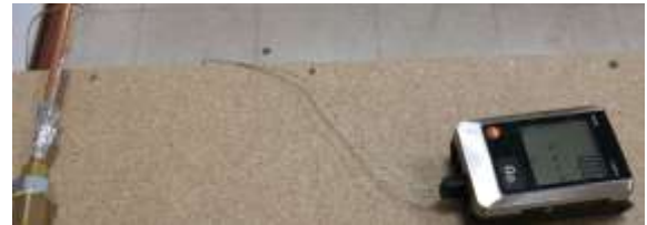
Figure 3. Temperature data logger
