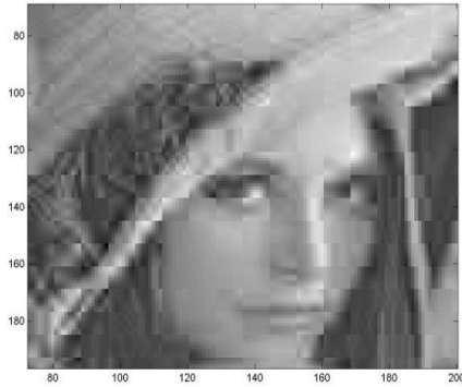
Figure 3. Blocking effect of DCT using 8 x 8 blocks.
