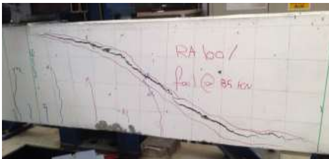
Fig. 2: Failure conditions of specimen 35-A-0-100
