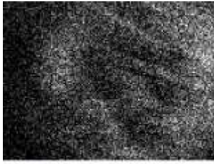
Figure 8: EDX Image for Aluminum
