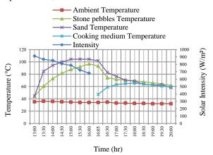
Figure 5: Variation of temperature and solar radiation intensity for transfer time of 05 minutes; September 16, 2014
