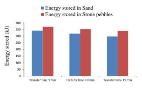
Figure 8: Heat stored by sensible heat storage materials
