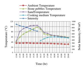
Figure 7: Variation of temperature and solar radiation intensity for transfer time of 15 minutes; September 23, 2014
