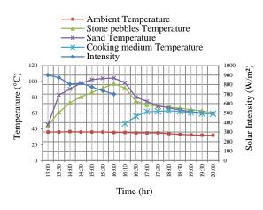
Figure 6: Variation of temperature and solar radiation intensity for transfer time of 10 minutes; September 22, 2014
