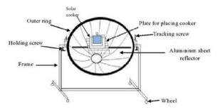
Figure 2: Schematic diagram of parabolic solar dish collector
