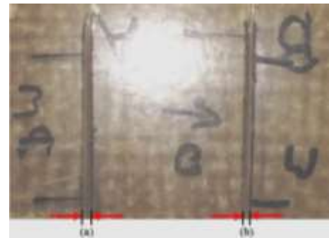
Figure 5: Top Kerf Width of machined GFRP specimen: (a) Free air (b) Under water
