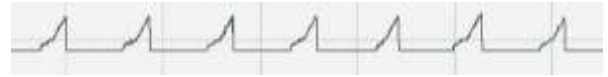
Figure 8: Current builds in the primary coil when the power transistor switched on.
