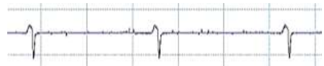
Figure 2: The signal pulse emitted by the crankshaft position sensor
