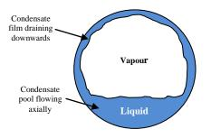
Figure 1. Condensation inside evaporator tube. (Wolverine Tube Inc 2006)
