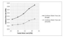
Figure 26. Condensate flow rate against feeder water load on both rough and smooth outer tube surface.
