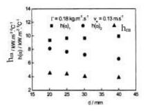
Figure 3. Effect of tube diameter, d on condensation side heat transfer coefficient, h(a)<sub>1</sub>, evaporation side heat transfer, h(a)<sub>2</sub> and total heat transfer coefficient, h<sub>m</sub>. (Xu et al. 2004a)
