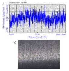
Figure 18. Surface roughness results on point P1 on smooth evaporator tube a) Ra  $(\mu m)=0.138,$  b) Surface profile (magnification 15 times)
