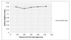
Figure 20. Overall surface roughness profiles on smooth tube.
