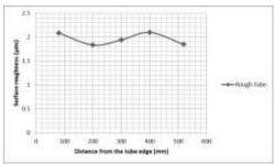
Figure 19. Overall surface roughness profiles on rough tube.
