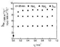
Figure 4. Effect of steam flow velocity, v<sub>s</sub> on condensation side heat transfer coefficient, h(a)<sub>1</sub>, evaporation side heat transfer, h(a)<sub>2</sub> and total heat transfer coefficient, h<sub>m</sub>. (Xu et al. 2004a)
