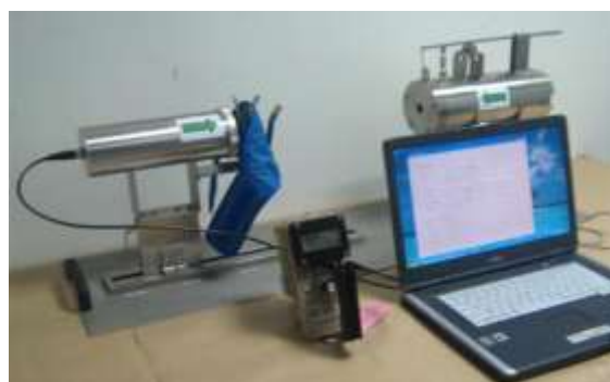
Fig. 1. A complete system of lead equivalent thickness gauge.
