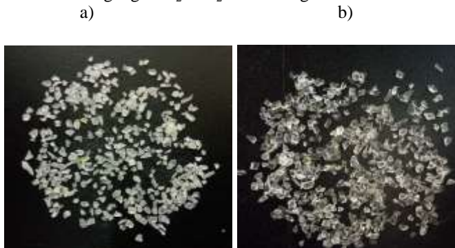
Figure 3. Glass beads before (a) and after (b) dip-coated with Ag-TiO 2 -SiO 2
