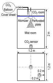
Figure 4. Test room for CO<sub>2</sub> adsorption by mist.
