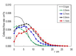
Figure 11. Comparison of radial distribution of droplets captured at 0.5 m below atomizer exit.
