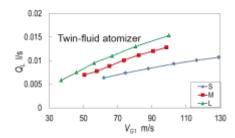
Figure 5. Mist flow rate against mean air velocity at twin-fluid atomizer inlet.
