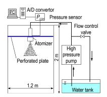
Figure 3. Test apparatus for the single-fluid type atomizer.
