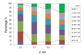
Figure 10. Effects of orifice diameter on droplet diameter composition for single-fluid 1 mm thick orifice type atomizers.
