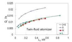
Figure 6. Comparison of mist flow rates among three atomizers S, M, L.
