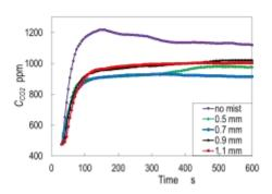
Figure 12. Time variation in CO<sub>2</sub> concentration in air at the bottom of mist room – Effects of orifice diameter in single-fluid 1 mm thick type atomizers.
