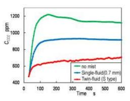
Figure 13. Time variation in  $CO_2$  concentration in air at the bottom of mist room – Effects of mists generated by a single-fluid type atomizer (1 mm thick orifice with 0.7 mm orifice diameter) and a twin-fluid S type atomizer.
