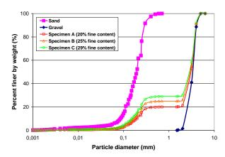
Figure 2. The particle size distribution of tested gradations
