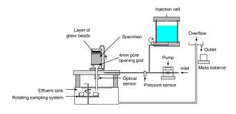
Figure 3. Schematic diagram of the erodimeter
