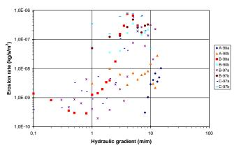
Figure 7. Variation of erosion rate to hydraulic gradient
