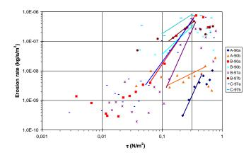
Figure 8. Variation of erosion rate to shear stress
