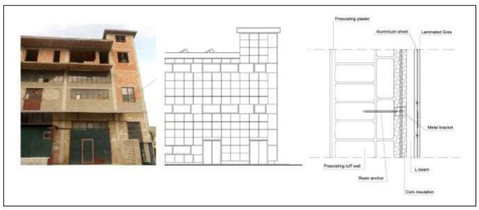
Figure 9. Left: part of the existing façade; centre: requalification of the façade with a ventilated wall; right: detail of the ventilated wall.
