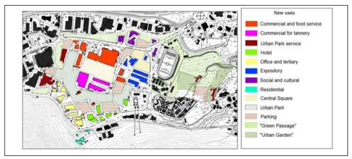
Figure 5. Possible requalification of macro area 3 with new uses (after demolition of several buildings)
