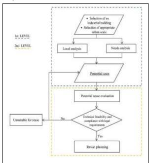
Figure 1. Flow-chart showing the proposed reuse methodology.
