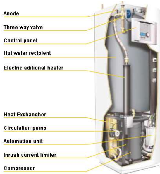
Fig.5 Heat Pump scheme (source: processed picture)
