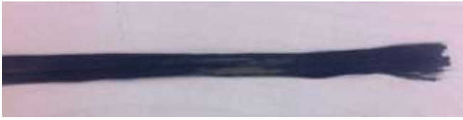
Figure 2. Carbon textile reinforcement uni-direction 50k.
