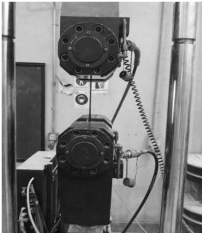
Figure 1. The setup of tensile test
