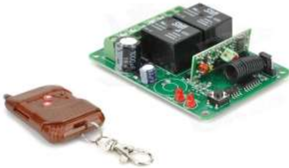
Figure 9. RF transmitter and receiver
