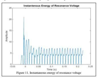
During the switching of power line instantaneous energy of voltage signal is increased approximately four times of the regular operation. After initiation signal has still two times of the regular operating state.
