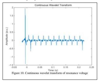
Some harmonic related transitions are displayed but most important of all the exact switching transition time can be detected with the corresponding amplitude value (2 p.u.). CWT signal transitions can reveal distinctive peak (resonance initiation) and point out system failure.
