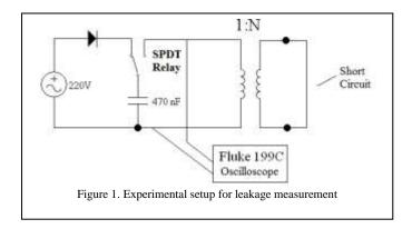
By calculating oscillation period, the leakage inductance is found as 3 mH. To predict non-linear B-H curve of transformer, input current and integral of voltage is displayed at dual trace oscilloscope with various input voltages (Fig. 2a). Here, Y channel corresponds integral of voltage and thus, flux linkage with 10x attenuation, and X channel corresponds to 1.6 times of current.
