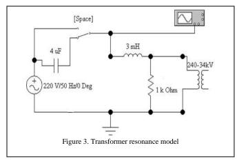
In simulation, initially, transformer is directly operated under system voltage. By pressing the space bar on the physical keyboard, SPDT switch changes its state and transformer is now in series with capacitor. Switching characteristics of the Low Voltage (LV) line is simulated by 4  $\mu F$  capacitor. A dry type 220V/34.5kV, 400VA, 50Hz test transformer, which is shown in Fig. 4 is employed to conduct real resonance tests.
