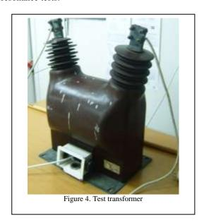
An autotransformer is used for connecting primary side of the test transformer with power network. All signal waveforms are displayed and recorded by Fluke 199C scope meter. During the tests 470nF and 820nF capacitance combinations are used for obtaining 5.54 $\mu$ F capacity to realize resonance. All capacitors are designed to operate under 400V which is nominal voltage with tolerance for LV side. The test set-up is given in Fig. 5.
