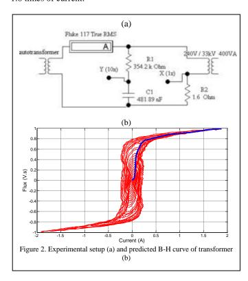
By using measured data, non-linear SPICE model of transformer is predicted by dividing B-H (Fig. 2b) curve into 15 coordinates which are obtained by different voltages supplied by autotransformer.
