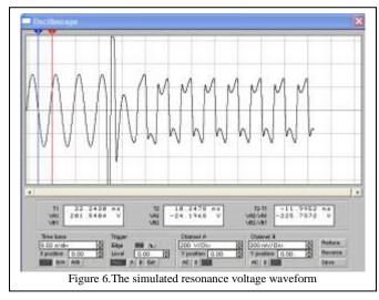
After initiation of resonance harmonics are observed on resonance voltage waveform. For this purpose FFT of voltage signal is analysed and frequency spectrum is given in Fig. 7.
