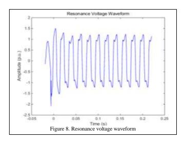
In order to reach proper comparison, frequency spectrum of the resonance voltage is given in Fig. 9. Frequency spectrum of test results depicts similar results obtained from simulation results. In accordance with previous results 3rd, 5th and 7th harmonics are observed.
