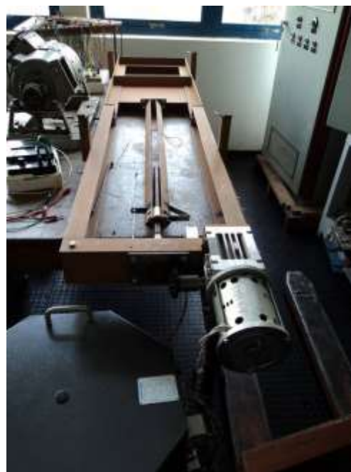
Figure 7: Hydraulic Floodgate and 24VDC motor.
