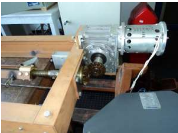
Figure 6: Hydraulic Floodgate 24VDC motor and speed reducer.
