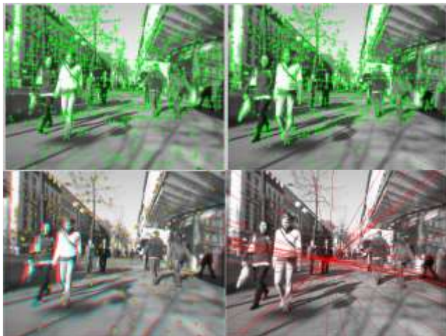
Figure 4. Egomotion estimation. Detected keypoints (green +) in frames i - 1 (top-left) and i (top-right) are matched (bottom-left) and egomotion is estimated using epipolar geometry (bottom-right). Here, only 30 sampled keypoints (red boxes) plus epipolar lines (red lines) are displayed for illustration.
