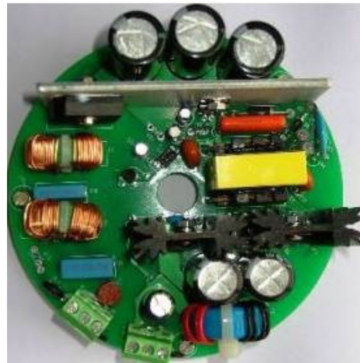
Fig 6. SMPS Power supply PCB
