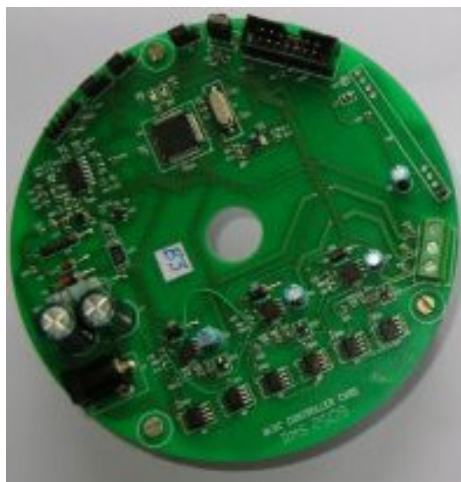
Fig 8. BLDC controller PCBA
