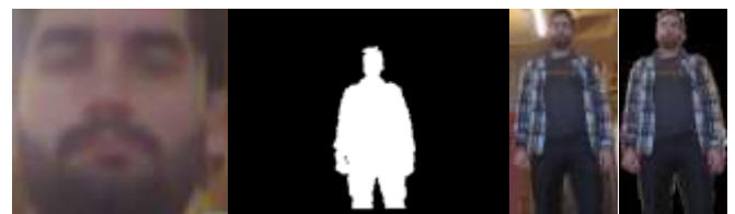
Figure 6. From left to right, extracted user's face, Boolean mask of the user, extracted user's body and extracted user's body with background removal.
