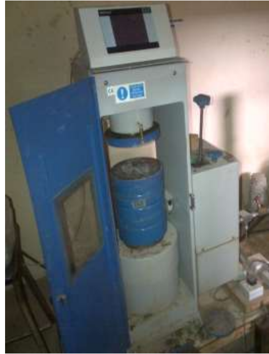
Plate 2.2 ADR Touch Compressive Testing
