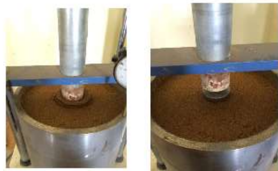
Fig. 6 soil footing system before and after load application
