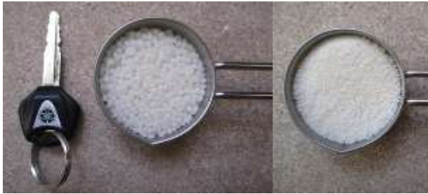
Figure 6. Fischer-Tropsch and Fatty acid amide wax
