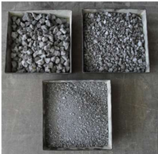
Figure 3. Black slag of EAF divided by size: 0/6; 6/12 and 12/18
