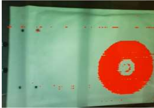
Fig. 4 The control monitor of the postal scanner. It shows a real time image of the envelope with CD disc inside. The envelope is moving on the control belt. Image is obtained by the fusion of the visible and 300 GHz images [12].
