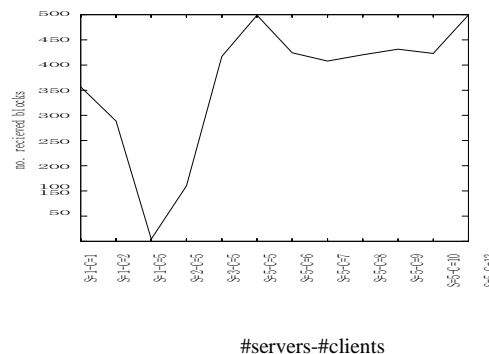
Fig. 3. Average number of received blocks in a time unit for a single client.
