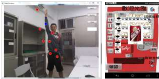
Figure 8. The gesture command “Lifting the right hand over the head” made by an action player for purchasing the sarsaparilla on the APP of vending machines of the smart device.
