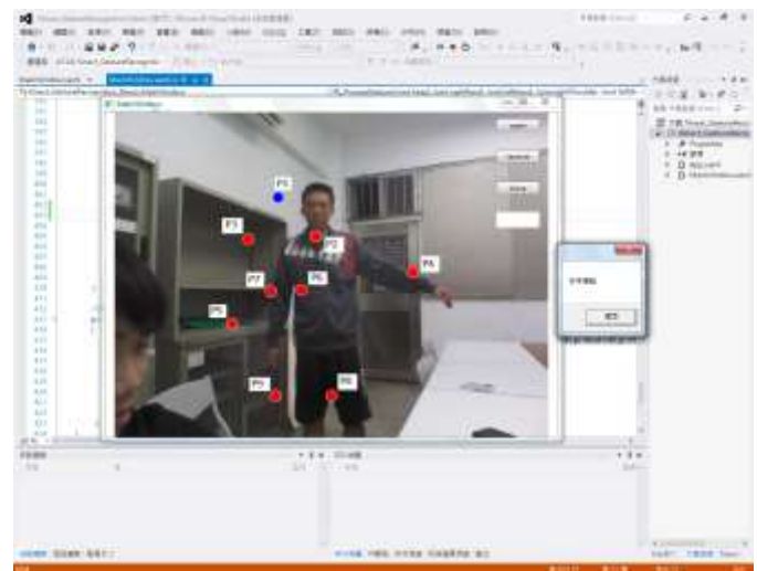
Figure 3. Feature-based Kinect SDK-gesture recognition using the spatial position information of kernel human joints (the gesture command “Waving the left-hand” operated by an action player)
