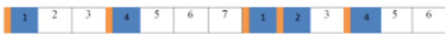
Fig 3: With Power Saver Slot. Slot 2 switches to sleep mode since no mobile node is detected by slot 1.
