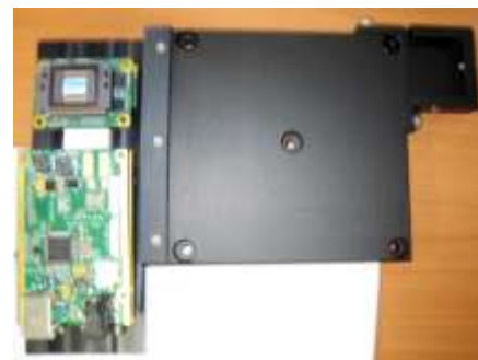
Figure 7 Chuck system for CCD Camera and standard specimen
