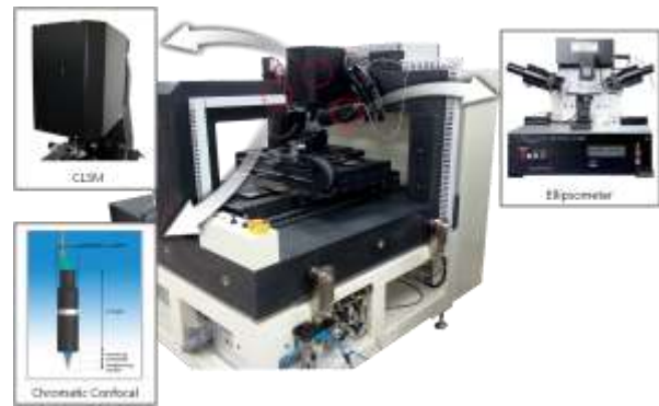
Fig. 10 Multi probe layout of measurement system
