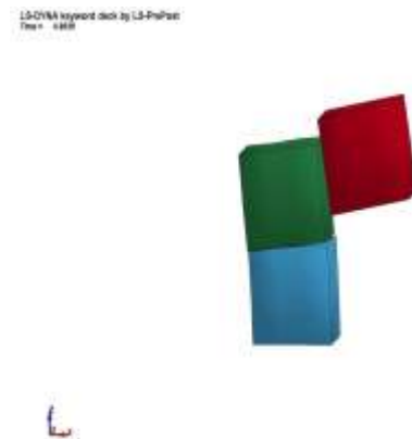
Figure 6. Block impact under breakaway conditions in the equation (1) (4.8 sec)
