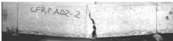
Figure 9. Flexural failure of CFRP/concrete beam with polyester mesh
