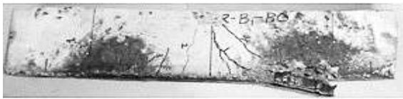
Figure 7. Cover separation failure of CFRP/concrete beam anchored with CFRP U wraps
