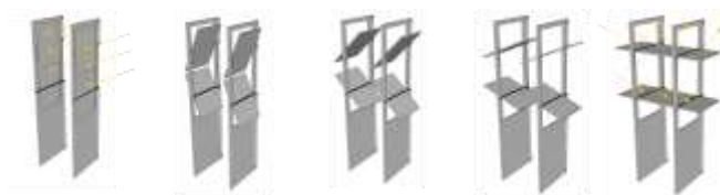
Figure 7. Transformation Procedure of the Proposed Façade System
