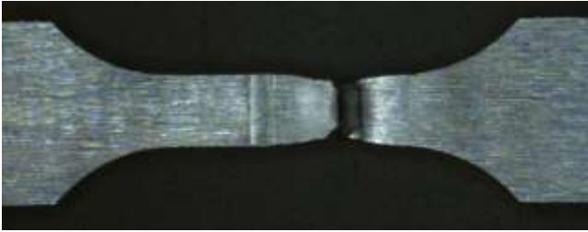
Figure 5 - Contraction of basic material outside the weld zone during the tensile test, position of the weld between the white lines
