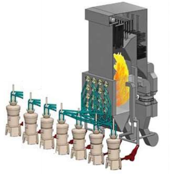
Figure 3. Coal mills that supply pulverized coal to the burners at different elevations.
