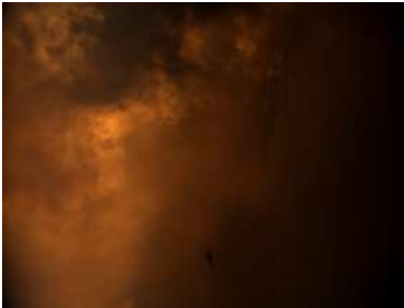
Figure 5. Raw flame image taken from one of the peek holes of the furnace.
