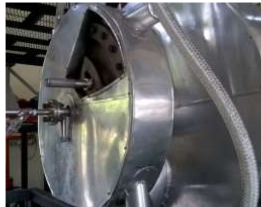
Figure 2. Swirl block for imparting swirling flows in the furnace of the combustion test rig.
