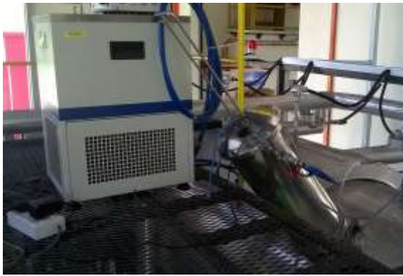
Figure 3. IR camera with water cooling system on the combustion test facility.
