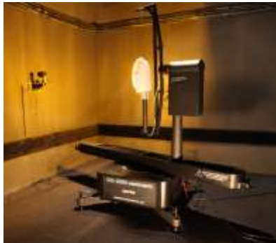
Fig. 2 Goniophotometer measurement setup
