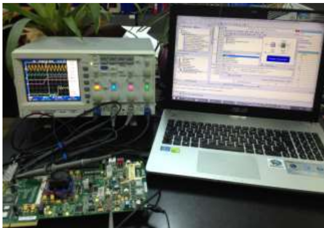
Figure 4. HT thread jitter measurement on nMPRA-MT processor using Virtex-6 FPGA ML605 Evaluation Kit – Xilinx.
