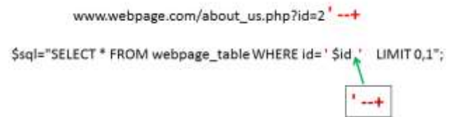
Figure 4. Inserting unauthorized character through user input
