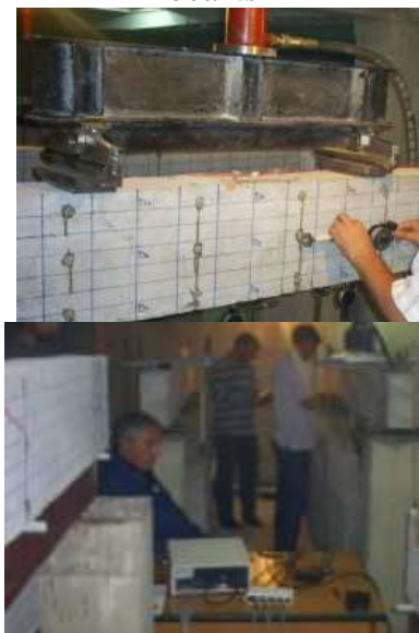
Fig. 3. Testing of beam in failure on the time t = 40 days- measuring of strains with mechanical and electronically strain gauges
