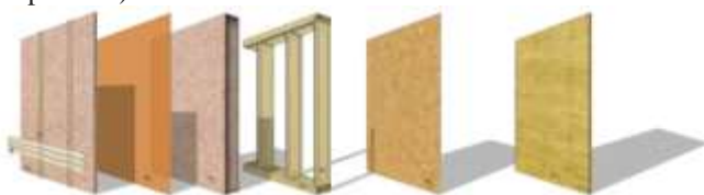
Figure 2 Platform frame and insulating layers
