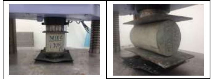
Figure 5. Compressive and split tensile strength test
