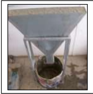
Figure 3. Experiment in progress for V-funnel test
