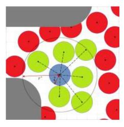
Figure 3. The performance of the proposed algorithm (PRM\*). Sampling and neighborhood radiuses are illustrated in a simple 2D environment. Current sample (blue circle) is being connected only to the neighbors within the neighborhood radius  $r^*(n)$  while the samples follow the sampling radius  $r^s(n)$  associated with the Poisson-disk sampling. Eligible neighbor nodes are depicted by green circles.
