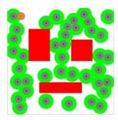
Figure 1. The implementation of the boundary sampling in a simple 2D environments with three obstacles. The new sample (orange circle) will be generates on the boundary of the union of forbidden region after the occurrence of the first rejection.
