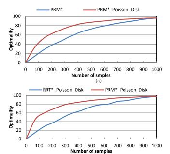
Figure 5. The minimum number of samples needed to reach different levels of optimality for (a) PRM\* and PRM\*\_Poisson\_Disk and (b) RRT\* and RRT\*\_Poisson\_Disk. The results are averaged over all seven cases presented in Figures 5 and 6 for 1000 iterations.
