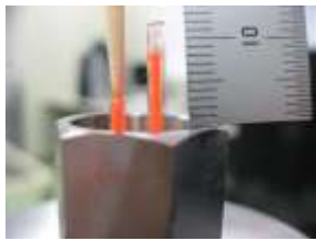
Fig.8 Measurement of liquid surface level
