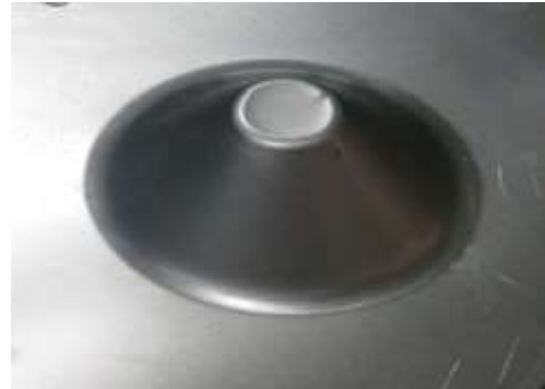
Figure 4. Formed conical part using SPIF
