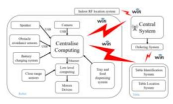
Figure 2: System Architecture
