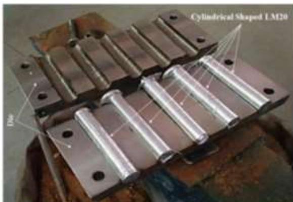
Figure 2. LM20 cylindrical shaped specimens
